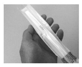
Next peel away the paper from the top to ensure that no wrinkles are created in the process. *If a wrinkle does occur simply pull down on the sheath to stretch the plastic around the lens.*
