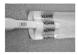
2. Slide the camera all the way to the end of the sheath until it releases from the wrapper. This will ensure a good tight fit.
