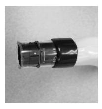
The camera is adjustable. Notice the two clear plastic rings around the lens. The top ring is the iris ring, which is used to control the brightness of the image. The bottom ring is the focus ring, which is used to focus the camera.
